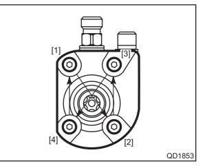
(4) Pull the element sub-assembly until it faces straight up and remove the element sub-assembly, plunger, and spring.
