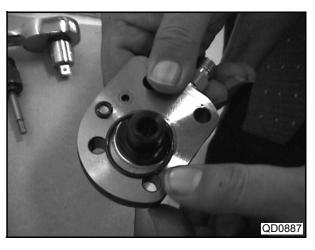
(7) Secure the pump as shown at right to remove the element sub-assembly on the opposite side.
