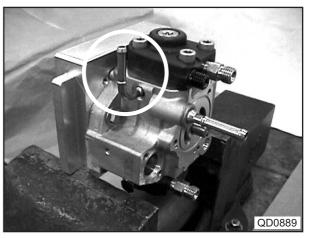
(8) Loosen the three hexagonal bolts on top of the element sub-assembly.
