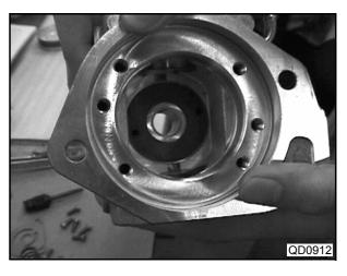
(4) Install the ring cam to the drive shaft.
