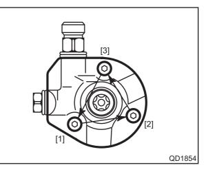
(9) Pull the element sub-assembly until it faces straight up and remove the element sub-assembly, plunger, and spring.
