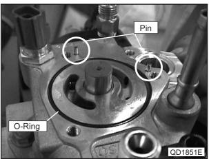
(4) Remove the O-ring and two pins.
