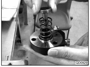
(7) Install the element sub-assembly assembled in step (6) to the pump body.
