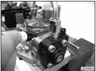
(2) Loosen the pipe nuts, and remove the pipes.
