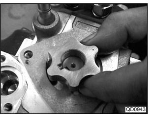
(6) Install the outer rotor.
