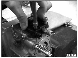
Please tighten the four hexagonal bolts uniformly in the order shown at right.
