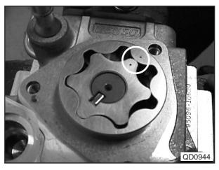
(7) Install an O-ring to the cover and the feed pump.
