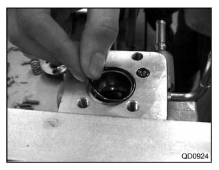
(3) Install the element sub-assembly assembled in step (1) to the pump body.
