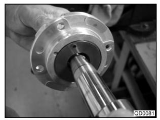
(3) Install the drive shaft in the cover sub-assembly.
