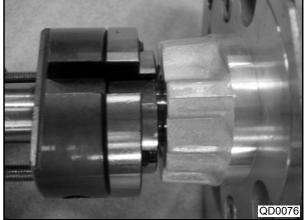
(7) Install the dial gauge on the camshaft clearance measurer.
