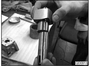
(5) Install the parts (drive shaft and ring cam) assembled in step (4) to the pump housing.
