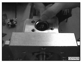
(6) Install the spring and plunger in the opposite side of the element sub-assembly.
