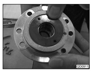
(2) Install a washer on the pump housing side as well.
