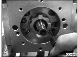
(2) Remove the key on top of the drive shaft.
