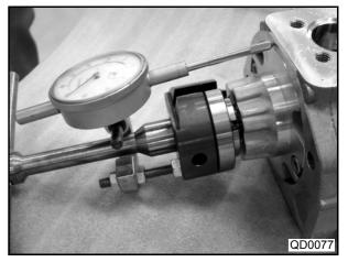
(8) Pull the camshaft clearance measurer to set the dial gauge to 0.
