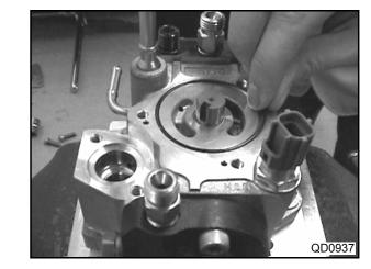
(2) Install position-holding pins in two places.
