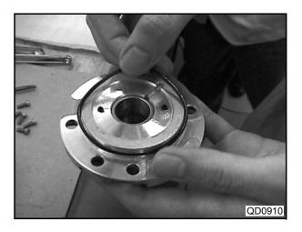
(2) Install the washer on the cover sub-assembly.
