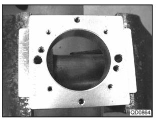
(2) Using two bolts, install the pump body on the pump plate assembly (STT).
