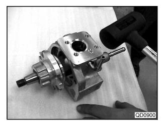
(6) Remove the drive shaft from the feed pump side.
