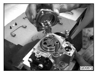
(2) Remove the feed pump rotor set.
