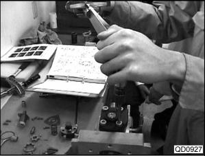
(5) Install an O-ring on the pump body on the opposite side of where the element sub-assembly will be installed.
