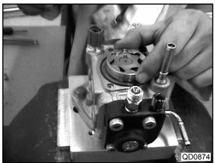
(3) Remove the feed pump plate.
