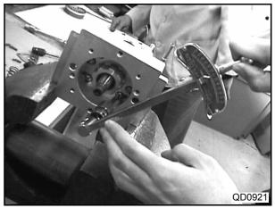
Please tighten the six hexagonal bolts uniformly in the order shown at right.
