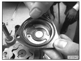
(8) Align the cover and the feed pump to the position-holding pins, and fasten them.
