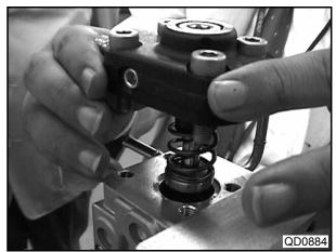
(5) Taking the plunger straight out of the element sub-assembly, remove the plunger and the spring.
