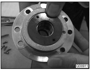
(3) Install a washer on the pump housing side as well.
